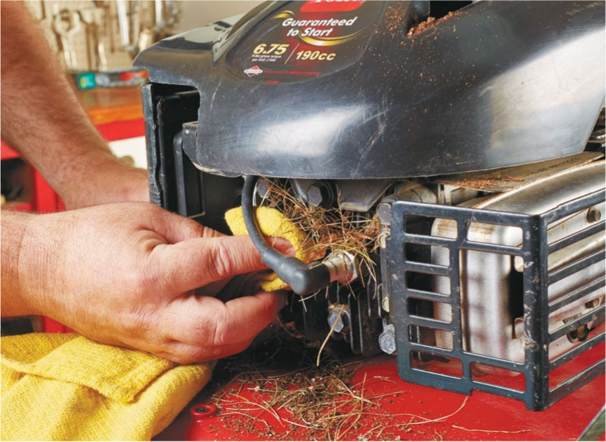
Cleaning off debris and gunk is a simple but critical part of any small-engine maintenance program.
